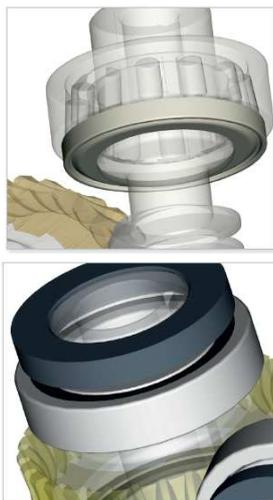
The combination on the input shaft of 2 taper roller bearings (mounted on size 75 and up to get an high resistance to the axial loads) and 2 nilos (mounted on the unit sizes 75 up to 150 to keep lubricating grease inside the bearings even when they are not touched by the lubrication oil) or, in alternative, special 2RS shields on such taper bearings, permits the mounting of the whole BOX range, from the size 25 to the size 150, in the positions V5 and V6.
